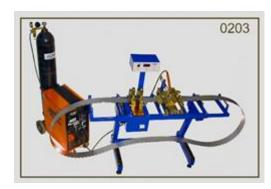
he unit is intended for electric arc welding of band saws with subsequent heat treatment of the seam. The installation is used in conjunction with a semi-automatic welding machine \*.
