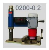
The grinding machine is an integral part of a set of equipment for the repair and manufacture of band saws from 20 to 50 mm wide. It is intended for processing a welded seam of band saws after welding. The grinder has a desktop version (attached to the table). The drive of the grinding stone from the electric motor, and the flow is carried out manually.
