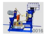
Installation allows for sharpening band saws in widths from 20 to 80 mm in increments of 8 to 38 mm with a tooth profile - "Sandvik", "Woodmizer", "Uddeholm", "Diamond", "Lenox" and the like. The installation has two performance options:
