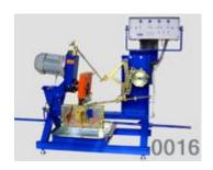
Installation allows for sharpening band saws in widths from 20 to 80 mm in increments of 8 to 38 mm with a tooth profile - "Sandvik", "Woodmizer", "Uddeholm", "Diamond", "Lenox" and the like. The installation has two performance options:
