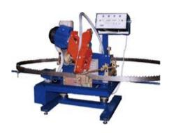
The installation of sharpening band saws is intended for sharpening the teeth of band saws, with the aim of obtaining a sharp cutting edge, as well as removing micro cracks along the entire tooth profile, by removing a thin layer of material by grinding. The unit uses profile borazon circles, which determines the shape of the saw tooth.
