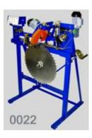
Sharpener is intended for sharpening of teeth of circular saws by method of dry grinding in the semi-automatic mode.
