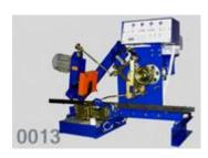
The unit is designed for sharpening band saws used in sawing wood, plywood, chipboard and fiber boards and other materials. The installation sharpens the entire tooth profile in order to obtain a sharp cutting edge, as well as removal of micro-cracks by removing the minimum amount of material throughout the tooth profile.
